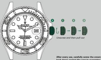
Arter every use, carefully screw the crown back down against the case to guarantee the waterproofness. Return the crown to position 1 and apply light pressure on it while screwing it down clockwise against the case. The crown should never be unscrewed underwater.
