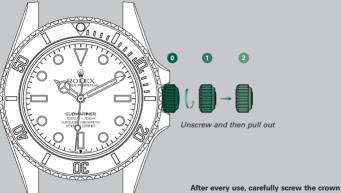
back down against the case to guarantee the waterproofness. Return the crown to position 1 and apply light pressure on it while screwing it down clockwise against the case. The crown should never be unscrewed underwater.
