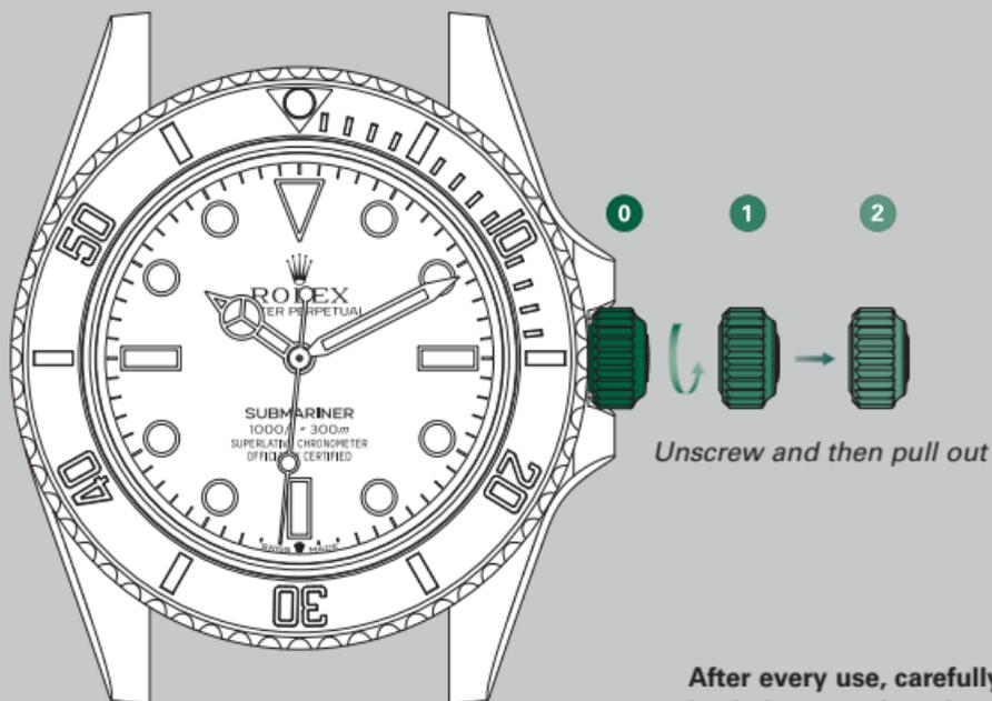
After every use, carefully screw the crown back down against the case to guarantee the waterproofness. Return the crown to *position 1* and apply light pressure on it while screwing it down clockwise against the case. The crown should never be unscrewed underwater.
