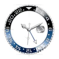
The Oyster Perpetual GMT-Master II allows travellers to simultaneously read their local time and reference (home) time. The former is indicated by the conventional hour, minute and seconds hands. The latter is indicated by the triangle-tipped 24-hour hand read against the graduations on the bezel when it is in the neutral position (triangle at 12 o'clock).
