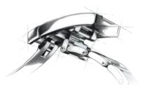
To ensure optimal comfort when wearing your watch in any circumstances, Rolex created the Easylink comfort extension link, which is available on some models. Its exclusive design, which was patented, allows the length of the bracelet to be adjusted by approximately 5 mm, without the use of tools.
