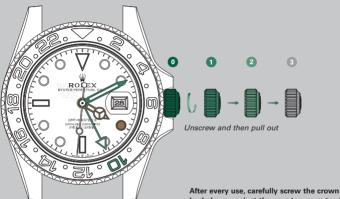
Arter every use, carefully screw the crown back down against the case to guarantee the waterproofness. Return the crown to position 1 and apply light pressure on it while screwing it down clockwise against the case. The crown should never be unscrewed underwater.
