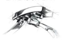
To ensure optimal comfort when wearing your watch, Rolex created the Easylink comfort extension link. This exclusive system comprises a link that is pulled out or folded back on itself to adjust the length of the bracelet by approximately 5 mm. without the need for tools.
