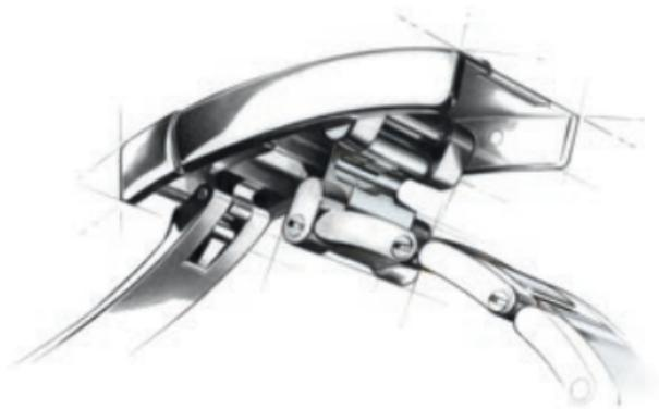
To ensure optimal comfort when wearing your watch, Rolex created the Easylink comfort extension link. Its exclusive design comprises a link that is pulled out or folded back on itself to adjust the length of the bracelet by approximately 5 mm, without the need for tools.
