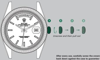
Anter every use, carefully screw the crown back down against the case to guarantee the waterproofness. Return the crown to position 1 and apply light pressure on it while screwing it down clockwise against the case. The crown should never be unscrewed underwater.
