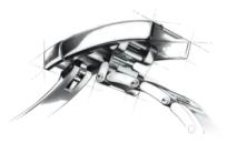
To ensure optimal comfort when wearing your watch, Rolex created the Easylink comfort extension link, which is available on some versions. Its exclusive design comprises a link that is pulled out or folded back on itself to adjust the length of the bracelet by approximately 5 mm, without the need for tools.
