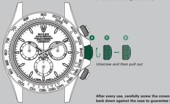
After every use, carefully screw the crown back down against the case to guarantee the waterproofness. Return the crown to *position 1* and apply light pressure on it while screwing it down clockwise against the case. The crown should never be unscrewed underwater.
