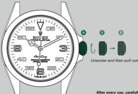
After every use, carefully screw the crown back down against the case to guarantee the waterproofness. Return the crown to *position* 1 and apply light pressure on it while screwing it down clockwise against the case. The crown should never be unscrewed underwater. ROLEX SERVICE
