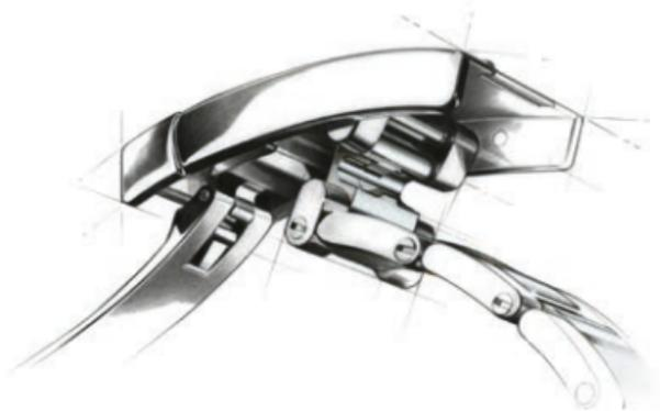
To ensure optimal comfort when wearing your watch, Rolex created the Easylink comfort extension link. Its exclusive design comprises a link that is pulled out or folded back on itself to adjust the length of the bracelet by approximately 5 mm, without the need for tools.
